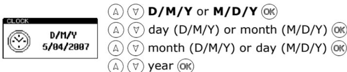
**TIP:** Pressing the **(\*)** button at any point will exit the clock set-up mode, leaving the time and date unchanged.
