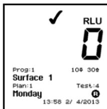
**NOTE:** Retest mode is automatically deselected once the new measurement is complete, or can be manually cancelled by pressing the **P** button and selecting a new program location.
