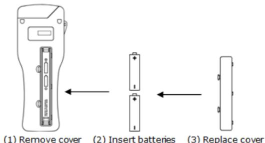
When the batteries are inserted correctly, the unit will automatically turn on and enter the clock set-up mode. (see section [3.8](#)).
