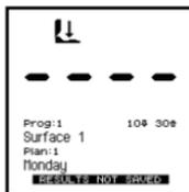
To change the Save Tests setting, select the **SAVE TESTS** menu option by pressing the **OK** button. Scroll to "SAVE TESTS" and press **OK** button to switch between ON and OFF:
