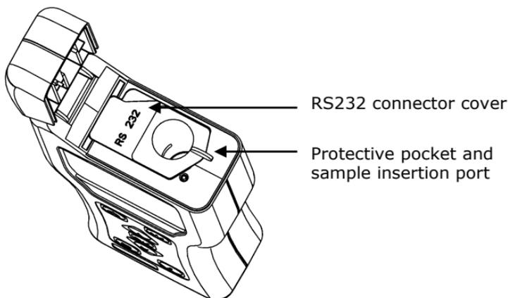
For details on the RS232/USB connector and protective pocket, refer to sections [5.6](#) and [6.1](#) respectively.
