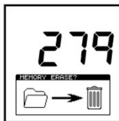
The entire test results memory can be cleared using the **MEMORY ERASE** function, by first selecting the **(\*)**, then using the up or down arrows to select the **MEMORY** menu option, then press **(OK)** to select, and then pressing and holding down the **(\*)** button for 2 seconds. The display will show the total number of stored results to be erased. To accept and start the erase function, press and hold down the **(OK)** button for 1 second, or press any other button to exit the option.
